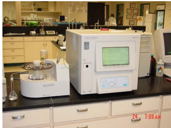
Total Organic Analyzer Unit at Polonio Pass Water Treatment Laboratory
