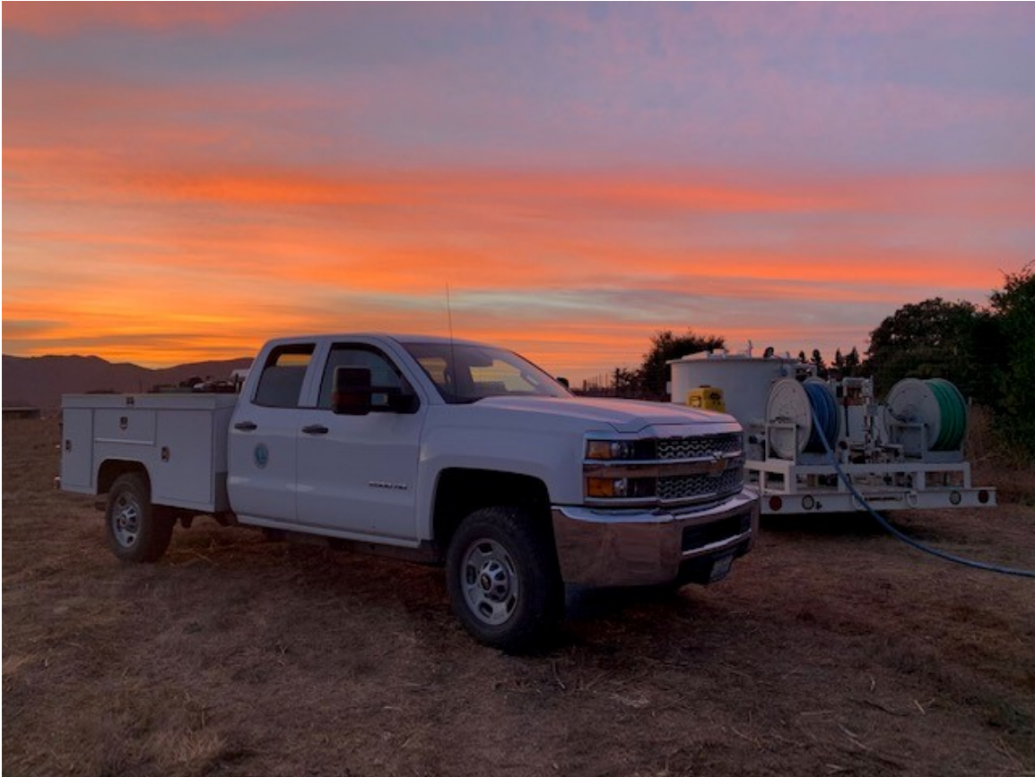
Distribution on Right of Way with de-chlorination trailer November 2020
