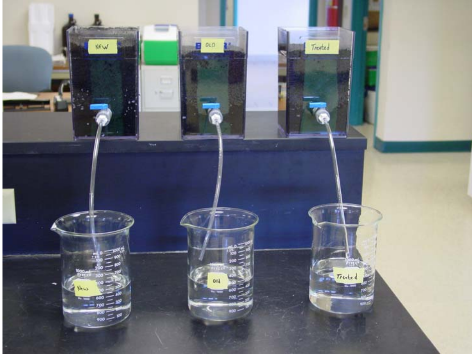
Bench scale granular activated carbon (GAC) tests were conducted to evaluate taste and odor removal capability.
